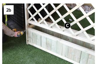
Locate Back Panel (C) onto side panels (B) and fix in position using 4x 90mm screws.
