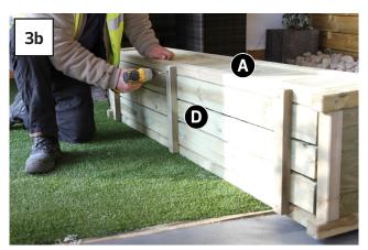
Position Base Panel (D) as shown and fix through battens using 6x 50mm screws.
