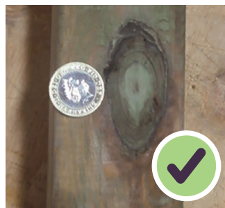
Knots are characteristics of timber.
