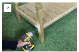
Place Shelf (C) between Leg Assemblies (B) and fix using 4 x 80mm Screws (1 x Screw per corner).
