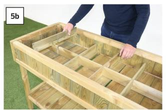
Place 1 x Long Divider (F) centrally between Side Panels (B) and interlock 4 x Short Dividers (G) as shown.
