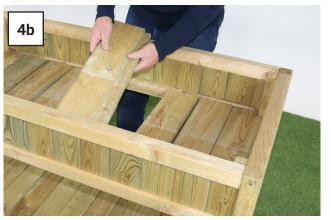
Locate 1 x Notched Slat (D) between Side Panels (A). Insert 7 x Slats (E) and remaining Notched Slat (D) between Side Panels (A). Ensure panels are equally spaced.
