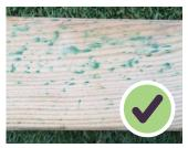
Most Zest products are pressure treated which protects the timber from rot for many years. Pressure treatment can result in a small amount of 'green spotting' on the surface of new timber caused by natural salts leaving the wood. This will fade away over time.
