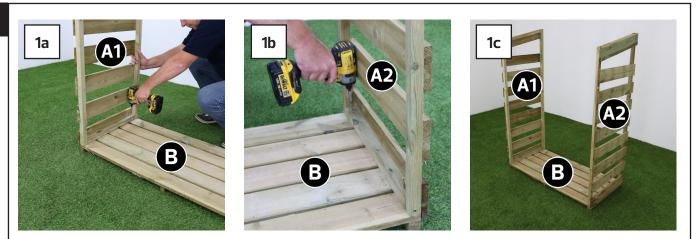
Locate Floor Board (B) and attach Side Panel (A1) and fix down using 2x 4x50mm screws 1 in each end as shown in above image. Repeat to fix the second Side Panel (A2) into the floor board again using 2x 4x50mm screws 1 in each end.
