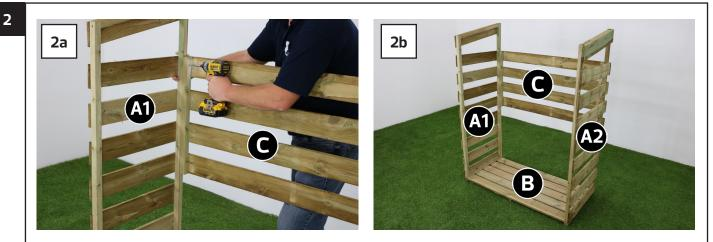
Fit Back Panel (C) to Side Panels (A1 & A2) using 2x 4x50mm screws on each side. Note: Align the back boards to the side boards as shown in above images.
