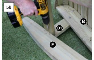
Locate seat legs into cut-outs in Rockers F and fix in position using 2no Screws for each of the rear legs (Fig.5a) and 3no Screws for each of the front legs (Fig.5b).
