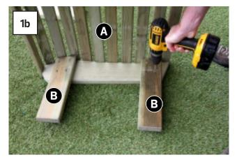
Position Legs B as shown in Figs.1a & 1b and attach to Stool Body A using 4no Screws per Leg. Repeat procedure for remaining Legs.
