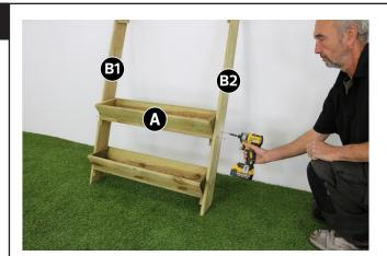
Place second Trough (A) onto subsequent battens and fix as described in instruction 1.
