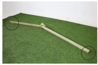
Attach angled end of 1x Rafter (F) to Finial Block (G) allowing a 20–25mm gap between Rafter (F) and Finial Block Capping using 1x 100mm Screw. Similarly attach 1x Rafter (F) to opposite side of Finial Block (G)
