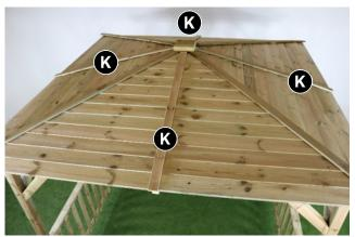
Position 1 x Short Cover Strip (K) centrally (angled cut beneath Finial Block capping and facing upwards) and fix using 6 x 45mm Screws, (2 x Screws per end and 2 x Screws to centre.) Repeat on remaining roof sections using 3 x Short Cover Strips (K)
