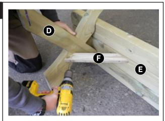
Attach Brace F to Bench Leg Assembly D and Seat E as shown using 2 x 70mm Screws. Repeat procedure for remaining Brace F.
