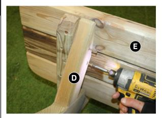
Attach Bench Leg Assembly D to the inside of outer battens of Seat E as shown using 3 x 80mm Screws. Repeat procedure for remaining Bench Leg Assembly D.
