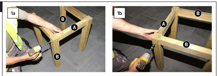
Attach Braces A to Legs Assembly B using 4 x 110mm Hex Screws (2 per Brace) as shown.
