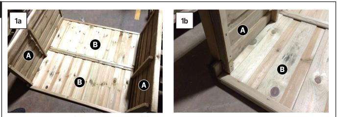
Set out Side Panels (A) and Back Panels (B) as shown in above and fix together using 6 x 60mm Screws – 3 per side.
