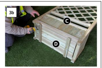
Position Base Panel (D) as shown in Fig 3a and fix through battens using 4no 60mm screws. See Fig 3b.
