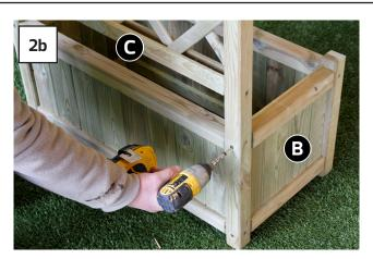
Locate Back Panel (C) onto Side Panels and fix in position using 4no 90mm screws. See Figs 2a & 2b.
