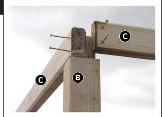
Position and fix Ring Beams C as shown in Fig. 2 using 4x 60mm screws (2 per beam). Repeat procedure for remaining posts and beams using 12x 60mm screws (4 per post).
